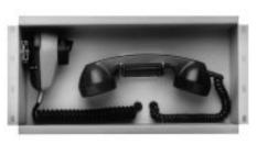
The NATIONAL TIME 900 Series Microphone/Telephone module encloses a paging microphone and firefighter's telephone. A microphone or telephone only enclosure is available by ordering A900-MIC or A900-TEL respectively. The enclosure mounts to the A900-FRAME and consumes 2 slots. Party line telephone and All Call microphone paging is possible with no additional modules. Zone paging and selective handset connection is provided when used in conjunction with the A900-CTRL MIC/TEL module.
